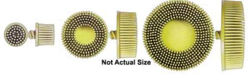
These Bristle Discs have abrasive grains embedded in the Bristles, the plastic breaks down exposing new abrasive as you use them, which makes them a great option for surface preparation, and removing gasket materials.
