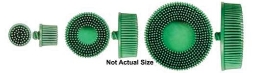
These Bristle Discs have abrasive grains embedded in the Bristles, the plastic breaks down exposing new abrasive as you use them, which makes them a great option for surface preparation, and removing gasket materials.
